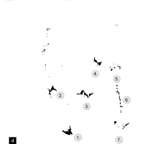
Fig. 5. The experimental results of proposed solution. (a) The frame captured from stereovision camera. (b) Disparity image; points being analyzed are marked with slanting lines; the darker color the further localized point; point for which disparity could not be calculated are marked white. (c) Potential obstacles points transformed to 2D map. Artifacts are visible. (d) Map of obstacles after spatial-time filtering.
