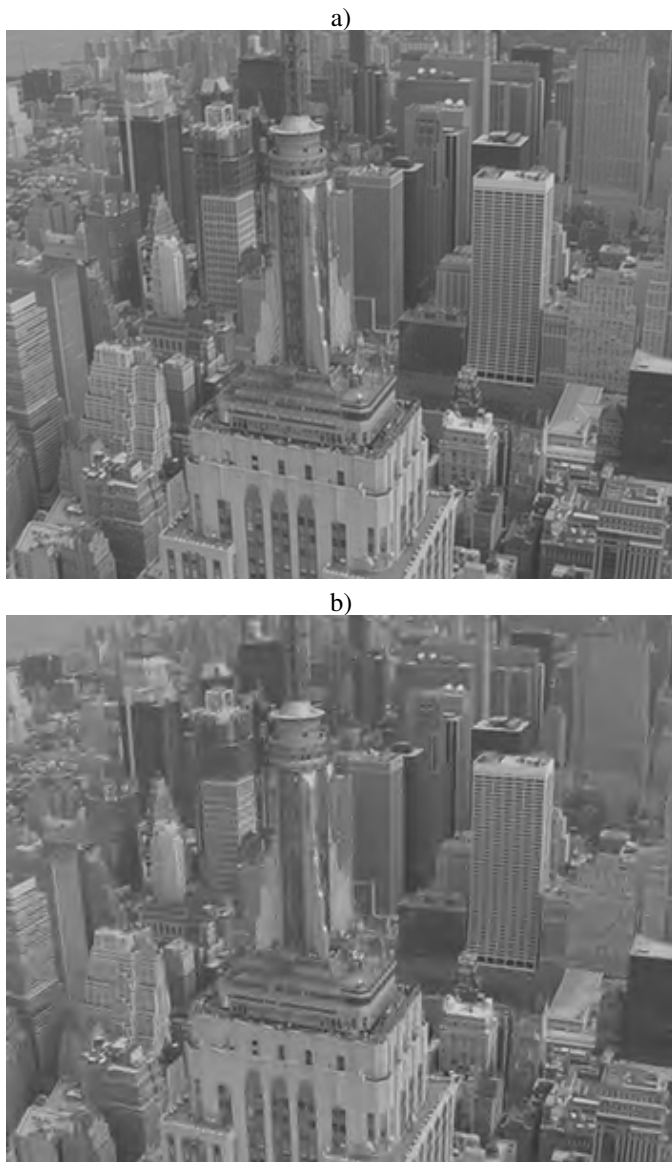
Fig. 6. A frame of the City video sequence a) for the longest coding time, PSNR=38.06dB, b) for the shortest coding time, PSNR=32.06dB; bitrate equal to 512kbps.
