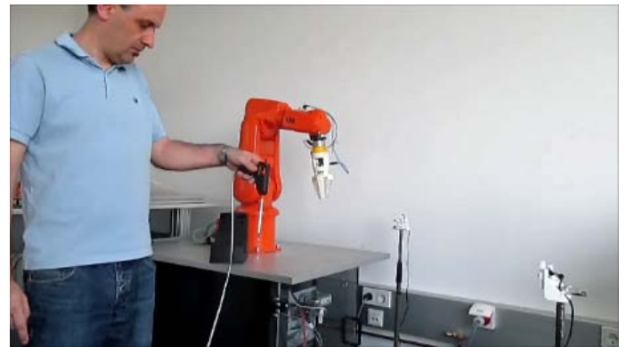
Fig. 10. Experimental set-up function test ABB IRB 120
