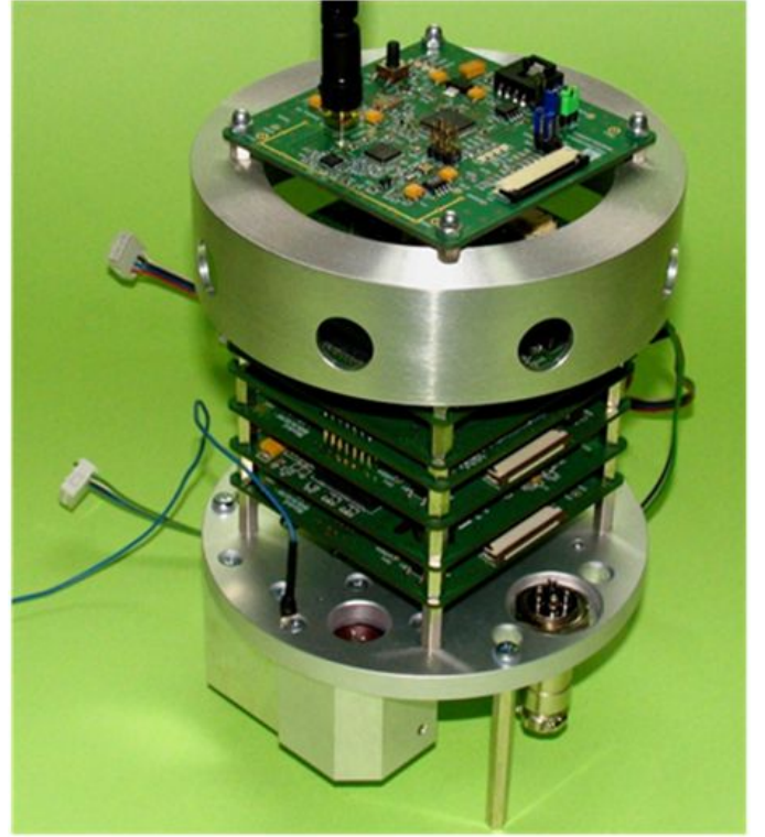
Fig. 2. The prototype of a seismic-acoustic sensor (with microphones removed). Three geophones have been mounted at the bottom of the sensor.
