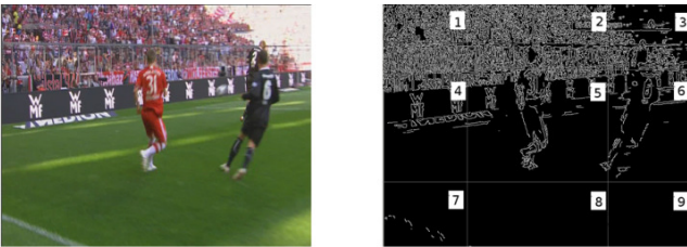
Fig. 16. The input frame and the mask as an output of the grass pixel ratio feature calculation.
