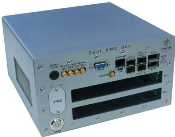
Fig. 4. Miniature MTCA case for two AMC modules [6]
