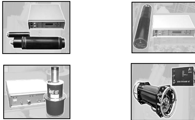
Figure 1. Compact neutron generators produced by VNIA. The upper pictures are vacuum tube based neutron generators and the bottom pictures are gas-filled tube based neutron generators [7] .
