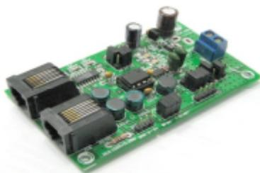
**Gambar 2.9** Modul DT-I/O NEO RS232 – RS485 converter
