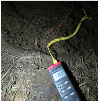
Figure 9. Thermocouple reading for third attempt at earth oven #2 (75cm wide/100cm deep).
