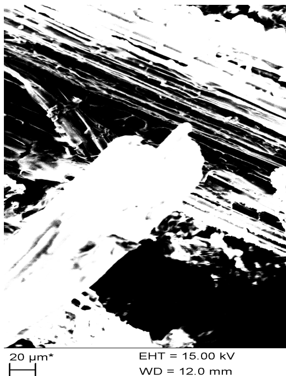
Figure 16: Sample after 9 hours pretreatment with [E(mim)]
