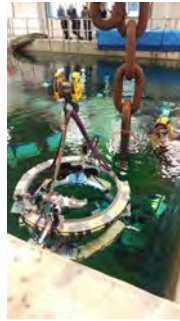
Step 2: Robot lowered into water tank
