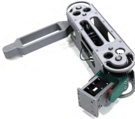
Fig. 7. The final manufactured leg. The initial aluminium parts were manufactured in FDM (PLA base) to reduce weight furthermore.
