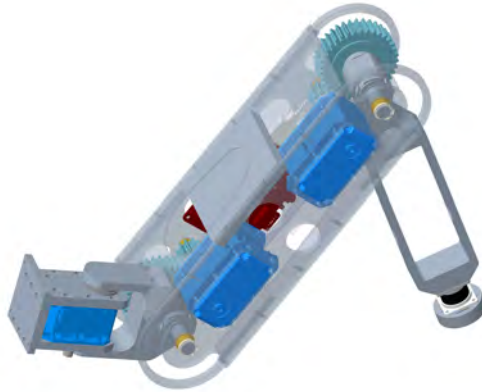
Fig. 6. A complete view of the robotic leg. The blue motors represent MX-106 model actuators. The dark red part is an integrated Raspberry Pi 3 for decentralized task handling.
