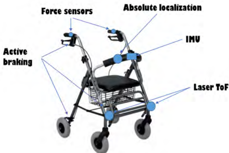
Figure 1. Block diagram of the installed systems on a commercial walker.
