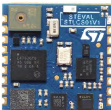
Figure 4. The sensorTile STLCS01V1 board.
