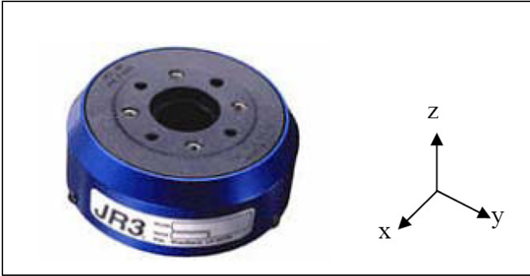
Figure 3.9 Six Axis Load Cell.
