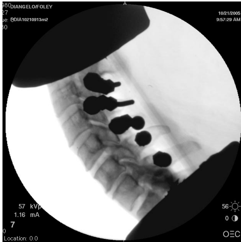
Figure 3.1 Specimen Evaluation. Radiographs such as the one above were taken and evaluated for specimen quality. These images are of specimen IU after the potting and rodding procedure.
