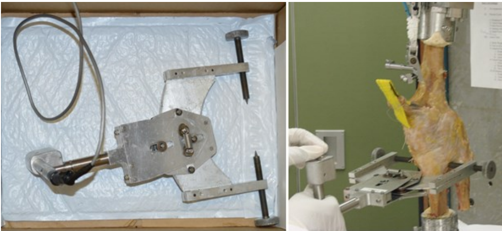
Figure 3-4: The arm attachment for quantifying anterior/posterior translation in TKA specimens. The other end of the cable attaches to a port on the front of the machine which transmits voltage readings associated with force and displacement. Force is directed perpendicular to the tibial axis.
