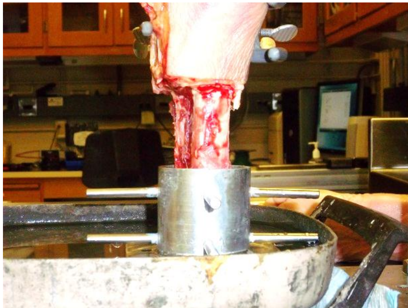
Figure 3-7. Potting specimen. Specimen aligned vertically in potting mold.
