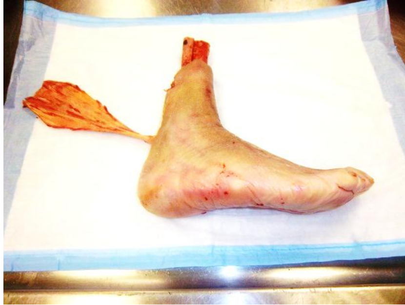
Figure 3-6. Dissecting tissue for testing. Tissue dissected to expose tibia/fibula, Achilles tendon, and the fibula being secured to the tibia.
