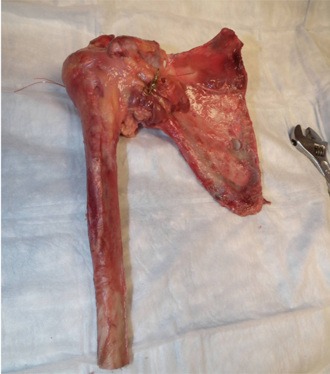
Figure 4-1. Photograph of the prepared GH joint specimen. Monofilament nylon was sutured into the humerus soft tissue at the origin of the RC muscles.
