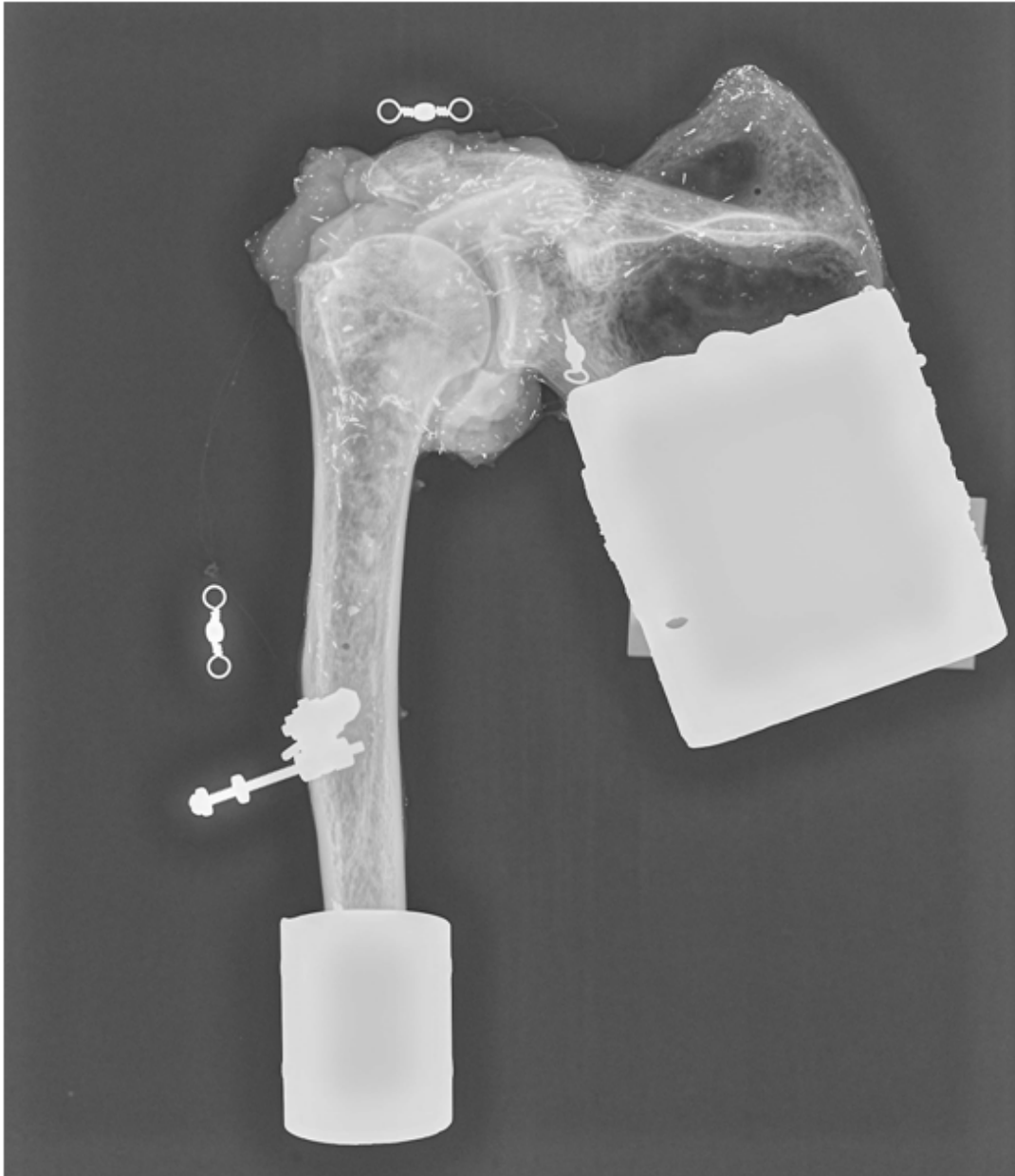
Figure A-1. Manual articulation specimen. Specimen has been potted, sutured and instrumented with a rod for 3D target placement.
