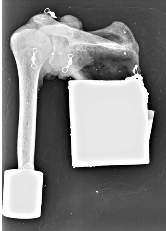
Figure A-2. Robot specimen. Specimen has been potted and sutured.
