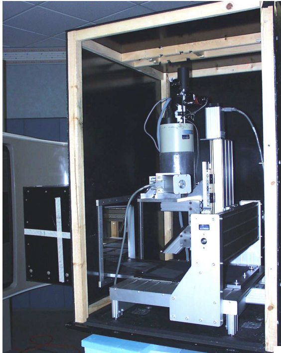
Figure 4-2.a CCD - CsI (Tl) portal imager assembly
