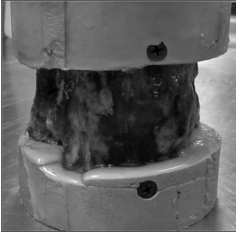
Figure 3-1 L4-L5 MSU Potted in Bismuth Alloy. The top and bottom plates are kept parallel to ensure repeatable mounting of the specimen.
