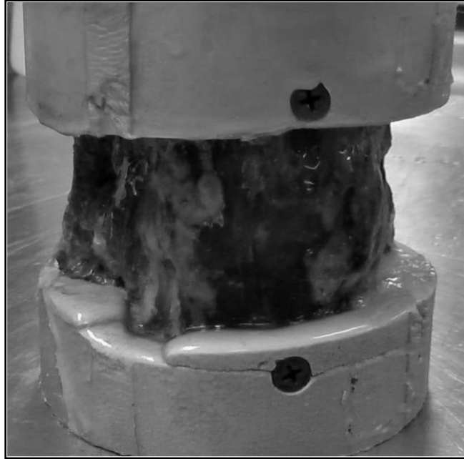
Figure 4-1 Potted L4-L5 MSU. The top and bottom plates are kept parallel to ensure repeatable mounting of the specimen.
