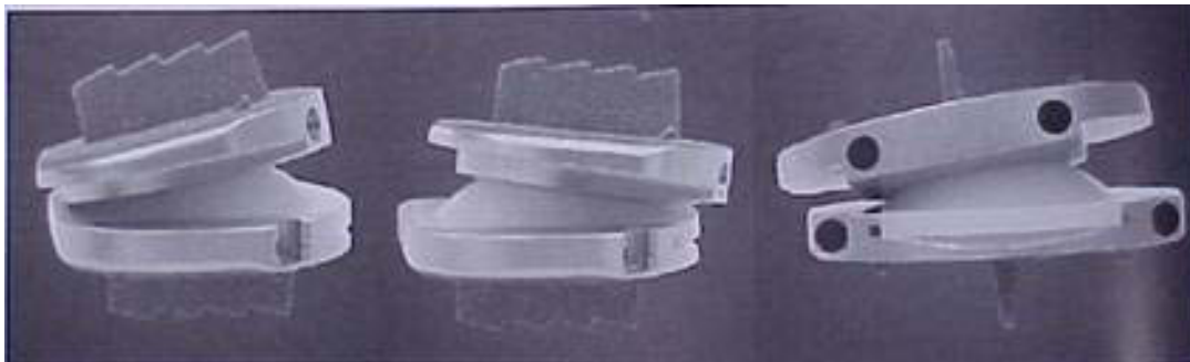
Figure 3-5: ProDisc-L Range of Motion. The ProDisc-L is a semi-constrained device that allows for rotations in all three planes and no translation. The center of rotation of the device is located centrally within the AP depth and offset a few millimeters below the endplate of the inferior plate.
