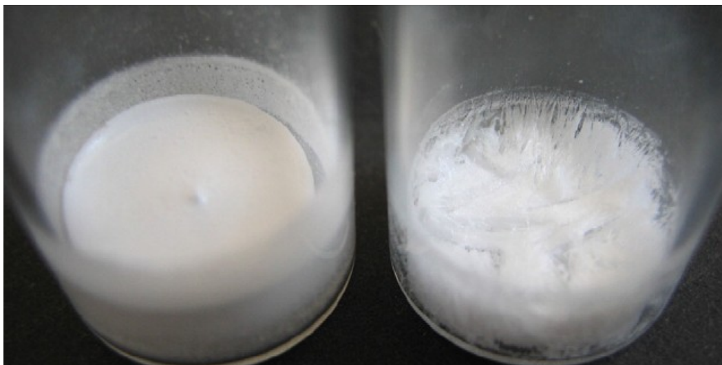
Figure 5.1 Representative samples of the MPS-L CRGD lyophilized with high (400 mM; left) and low (50 mM; right) concentrations of trehalose.
