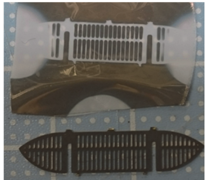
Fig. 3 Optical images of metal mask and sputtered Au pattern on the PC membrane.
