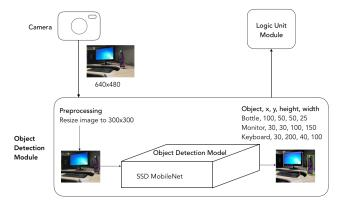
*Fig. 2:* Object detection module overview. Once the camera takes a snapshot of the scene, the image is passed to the object detection module. First, preprocessing is done, such as re-sizing the image to 300x300. Then, the preprocessed image is sent to an object detection model where the most probable object type and bounding box of each object are determined for each object. The object types and corresponding bounding boxes are then sent to the logic unit module.
