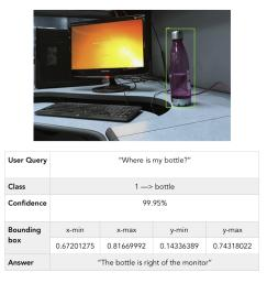
*Fig. 4:* Proof-of-concept OLIV system. In this example, the user asks "Where is my bottle?". Based on the detected 'bottle' object and its location (shown by a green bounding box) and its location relative to the landmark object (in this case, it is a stationary monitor), the semantic description response verbally conveyed to the user is "The bottle is right of the monitor".
