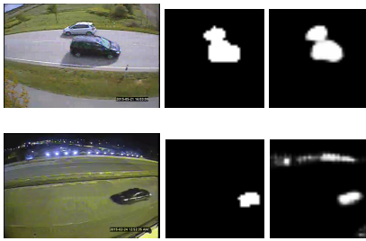
Fig. 4: Left: Input RGB images. Middle: human annotated vehicle mask. Right: vehicle detector probability map. In the top (bottom) image, the vehicle detector has an F_1 score of 0.89 (0.34). The blurry nighttime scene with bright lights is a case where this vehicle detector produces a number of false positives. The FDM predicts \tilde{F}_1 of 0.82 (0.36) for these, capturing the ground truth quite closely.
