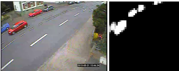
Fig. 1: Left: a typical road scene with 6 vehicles. Right: the output of our vehicle detector.
