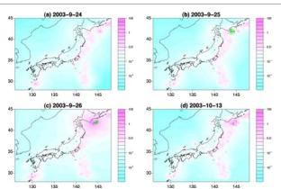
Examples of forecasted images of expected numbers of earthquakes on (a) 24 September 2003, (b) 25 September 2003, (c) 26 September 2003 and (d) 13 October 2003. (unit: events/day/deg $^2$ ). The green circles mark the locations of earthquakes  $(M_J \ge 4.0)$  occurring in forecasting time period.
