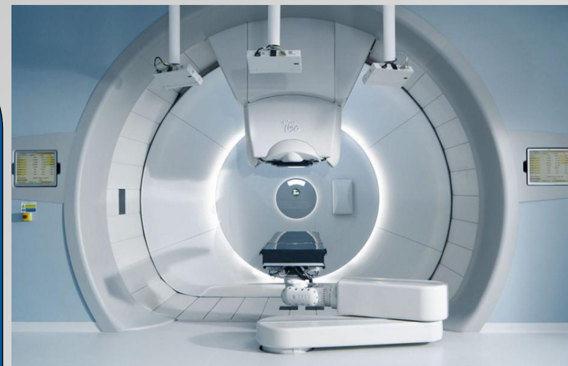
Fig. 1 (left): Gantry rotates 360° around the patient, delivering dose at any angle necessary.
