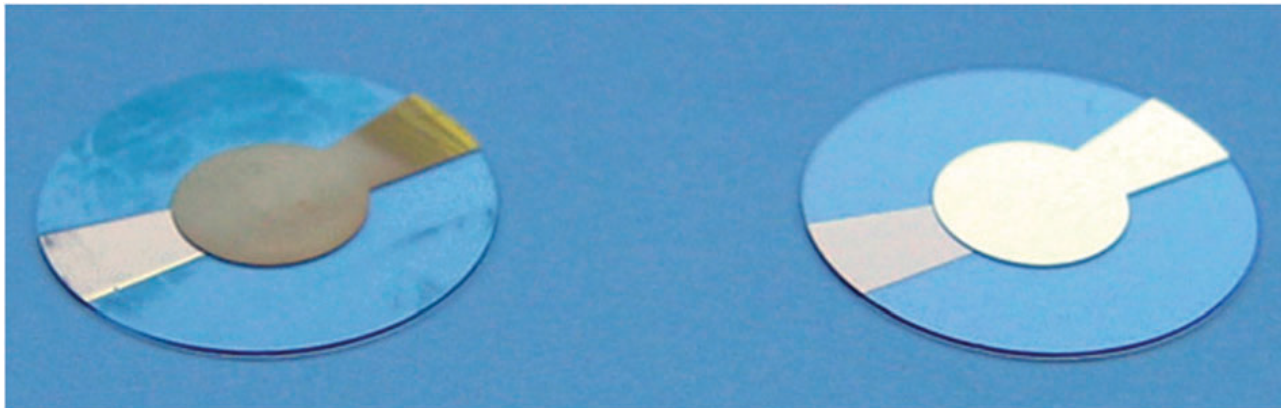
QCM-devices after growth of \text{Cu}_3(\text{btc})_2(\text{H}_2\text{O})_3 \cdot x\text{H}_2\text{O} : opaque layer on the SAM-modified gold electrode (left); reference chip without SAM on the gold surface (right).
