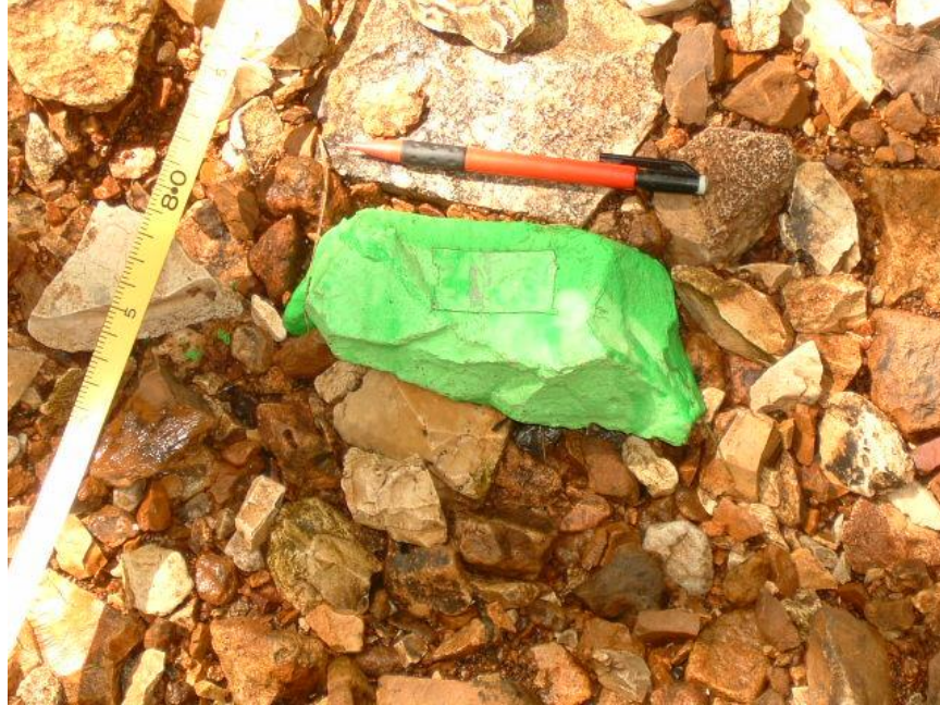
Picture 5: Sediment tracer recovery
