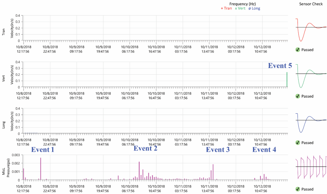
Figure 6. Output from the InstanTel Blastmate seismic and sound recorder: October 8 to 12, 2018. The bottom graphs show seismic events on the vertical (vert), transverse (Tran) and longitudinal (Long) components in in/s, and the sound events from the linear microphone (MicL) in psi. Three significant events are marked on the graphs.
