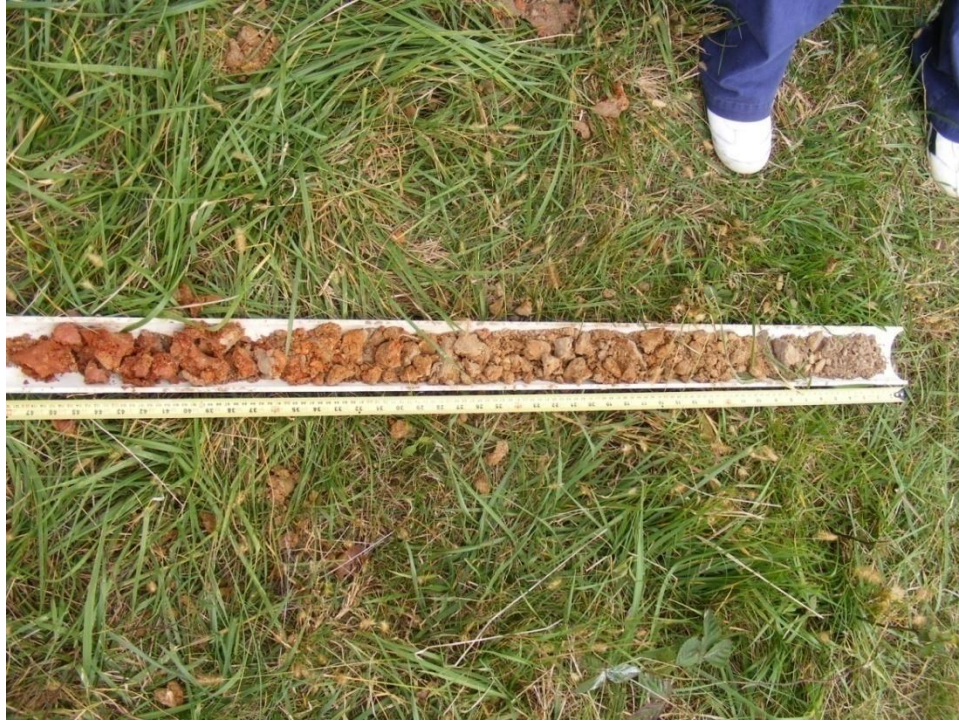
Photo 7. Example of a Soil Profile at the Project Site (Loess over Colluvium over Residuum) (October 2008)
