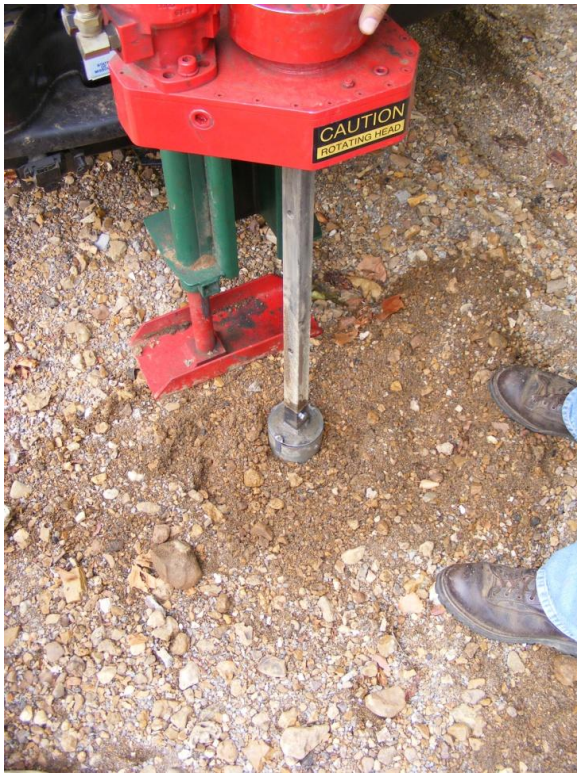
Figure 6B: Bar coring Bucket auger moving through bar material
