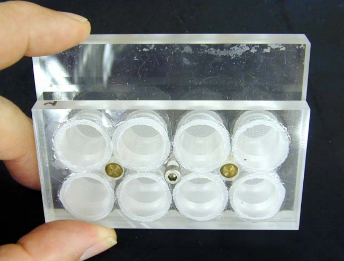
Figure 1. Container for hypoxia experiments. Similar units were placed at each of 6 different levels of dissolved oxygen in a flowing system. The facing plate is removable for placing juveniles in the compartments and for observations. The compartments are bounded on both ends by nylon screen to allow water to pass through.
