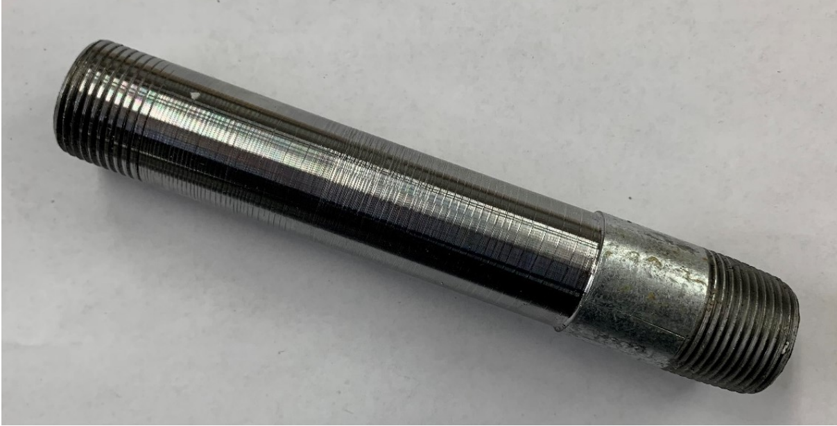
Appendix A-2. The nipple after 4.5" (11.4 cm) of its length has been machined down to a 1" (2.5 cm) outside diameter.
