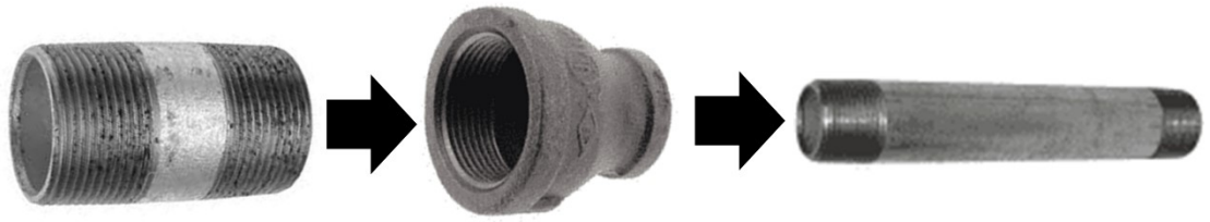
Appendix A-1. Pipe fittings that make up the coupling system (not to scale). From left to right, the 1 ¼" to 1 ¼" (3.175 cm) galvanized pipe nipple, the 1 ¼" to ¾" (1.9 cm) galvanized pipe reducing coupler, and the 6" (15.24 cm) in length ¾" to ¾" galvanized pipe nipple
