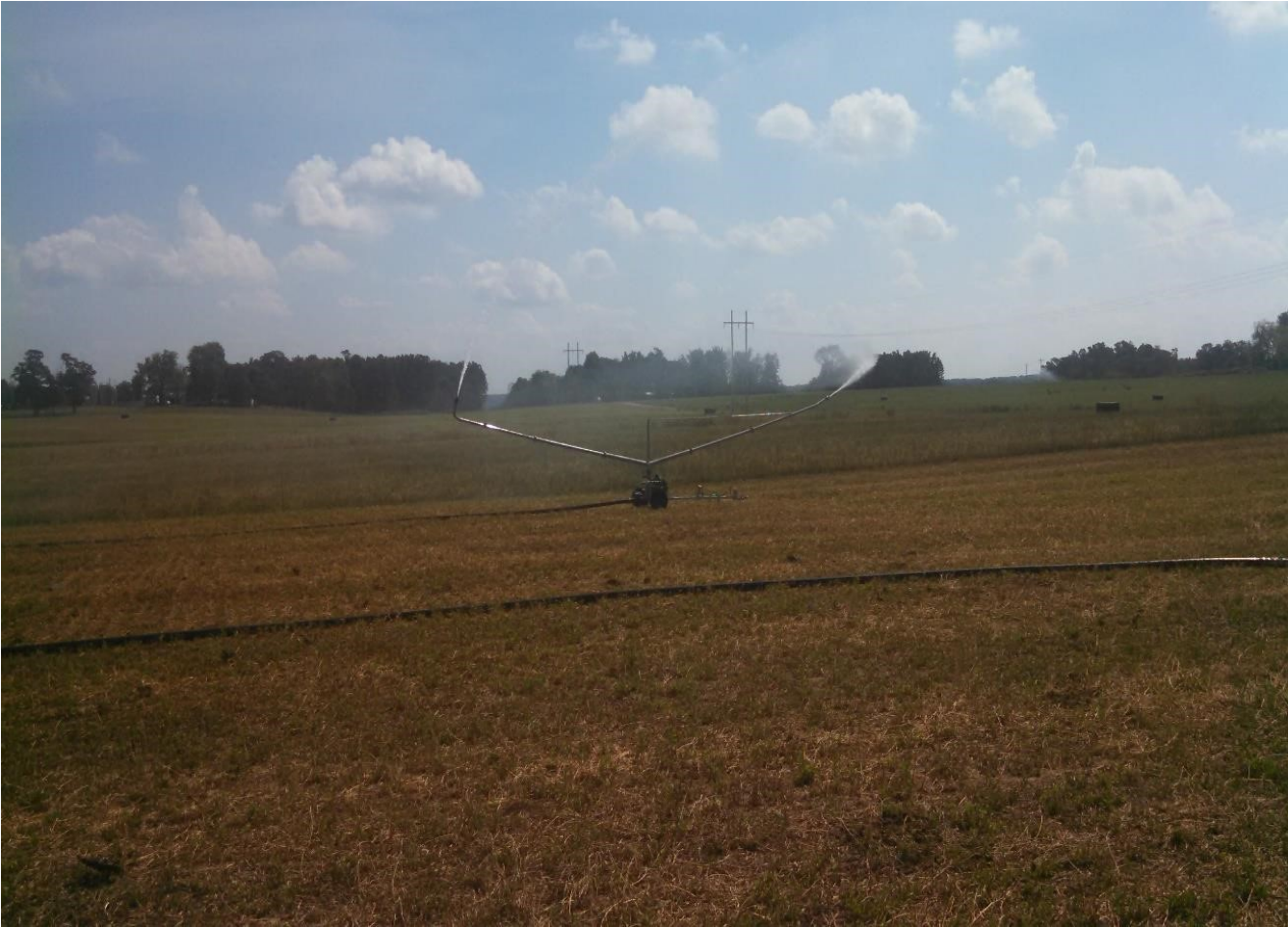
Figure 3. Low pressure traveling gun irrigation system located at Fletcher farm deployed on alfalfa paddock shortly after grazing event in September of 2016.
