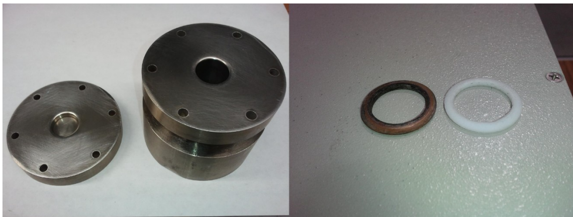
Figure 4. The hydrothermal reactor and gaskets. On the left is the hydrothermal reactor. The reactor is made of Hastelloy C-276 alloy. On the right, the two gaskets used for sealing between the reactor and lid.
