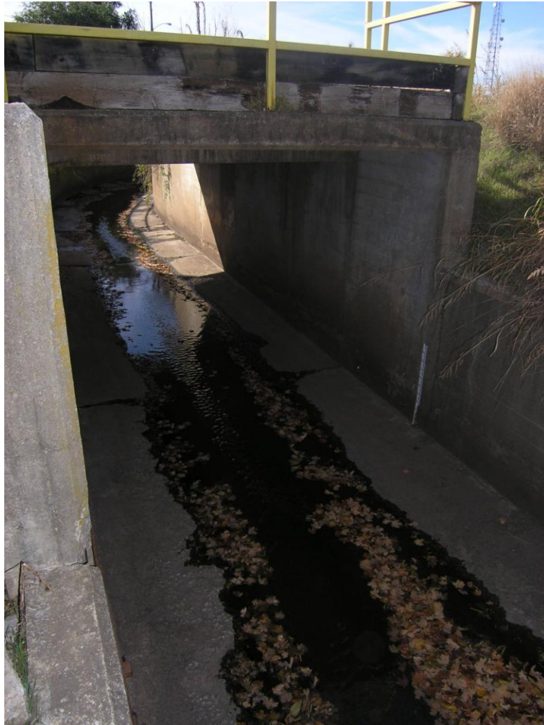
Site SB2 (South Branch Jordan at Hammons Parkway): Downstream view showing gage location and base flow. Base flow stream gaging was done at channel center and event stages were reported as staff gage reading plus elevation difference between gage base and channel center.
