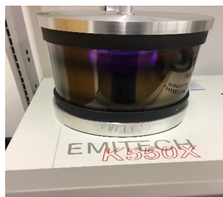
1 min Ar+O 2 plasma cleaning followed by a 30 sec Ar cleaning only
