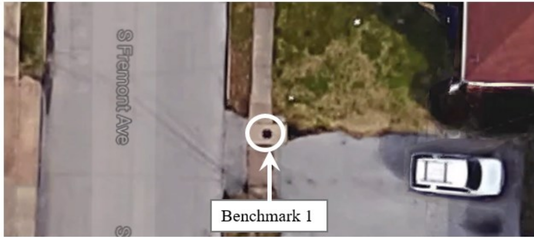
Figure 8. Sample benchmark selected for smartphone's GPS error calculation
