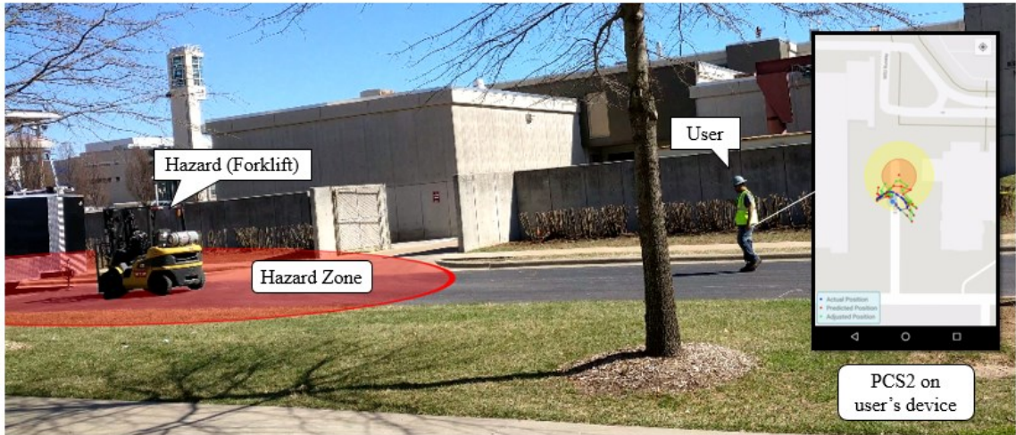
Figure 42. Experiment setup with the forklift as a site hazard
