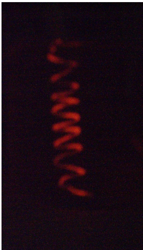
Figure 2. ECL emission of [\text{Ru}(\text{bpy})_3]^{2+} at a platinum electrode. Stirred solution of 0.15 M [\text{Ru}(\text{bpy})_3]^{2+} and 40 mM TPrA in 0.18 M potassium phosphate buffer (KPB) pH 8.0. Working electrode held at +2.0 V vs. Ag/AgCl. Photograph by D.J. Vinyard. 27 Jan. 2008.
