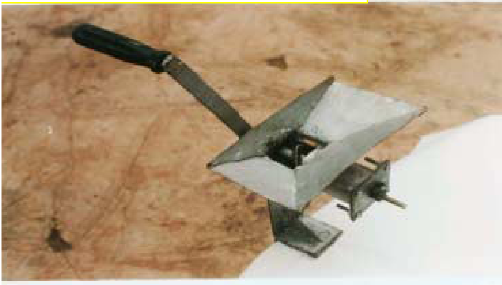
Plate 1 (a) Dough-dicing machine
