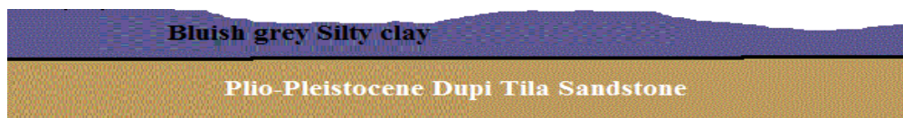
Figure 2: The hypothetical diagram showing the sediment deposits of the Plio-Pleistocene time which comprises of sandstone and overlain by the Holocene bluish grey silty clay. This bluish grey silty clay is the base of peat.
