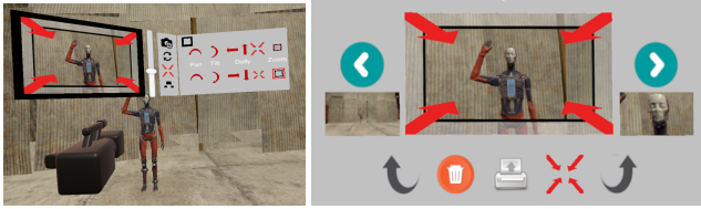
Figure 6: Our storyboard interface. (Left) A camera manipulator used to define the shot, the camera focal length and specify the type of camera motion. (Right) The 3D panel used to preview and organize the created shots.
