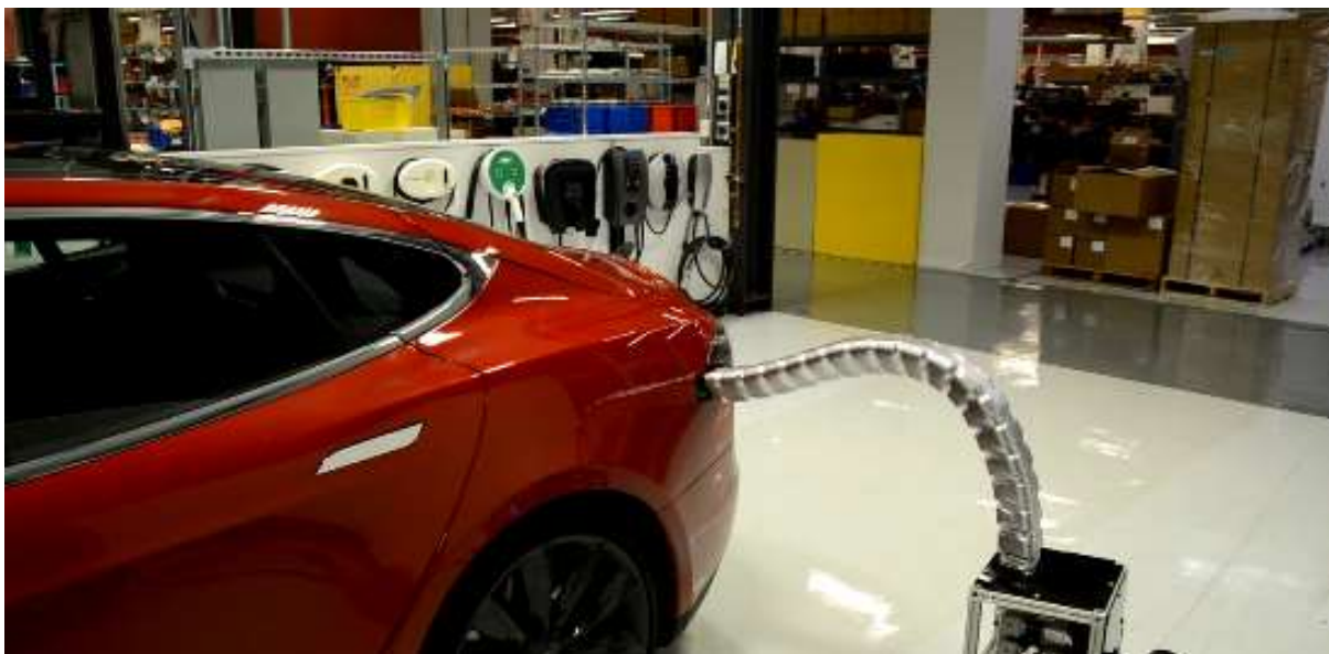
Figure 3. Tesla's "Solid Metal Snake" automated charging station prototype. (Tesla, 2015).
