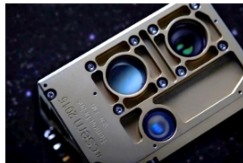
Fig. 8: Vision-based sensor (VBN). Top right: color camera optics. Bottom center: laser illumination head and above LiDAR receiver optics.
