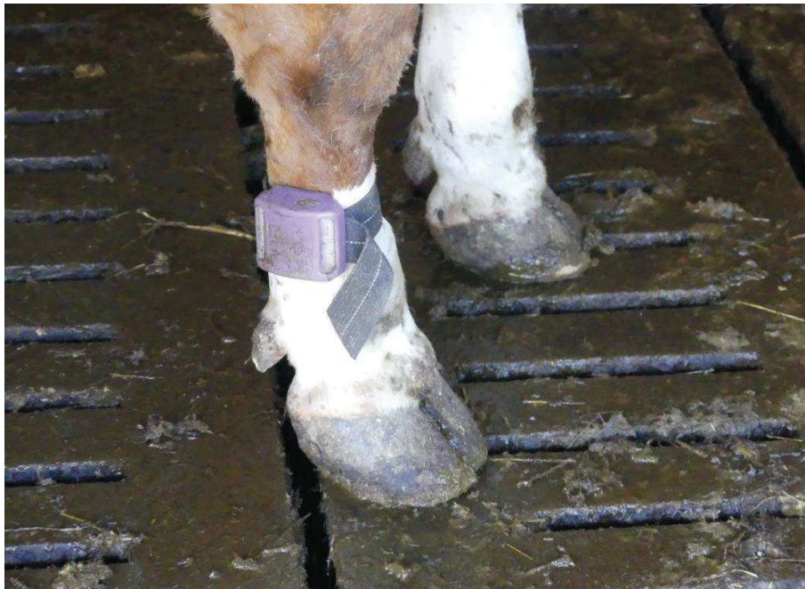
Figure 14: “Track a Cow” pedometer on the right front limb of a dairy cow
