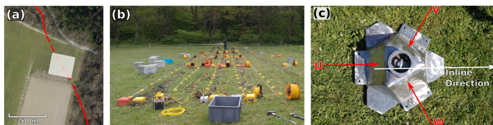
Figure 1: The basemap of Ettlingen Line; solid red line depicts the existing location of the trench line, dashed red line represent the buried site (a). 3D seismic acquisition using 3 component receiver (b) and 3 direction Galperin source (c).
