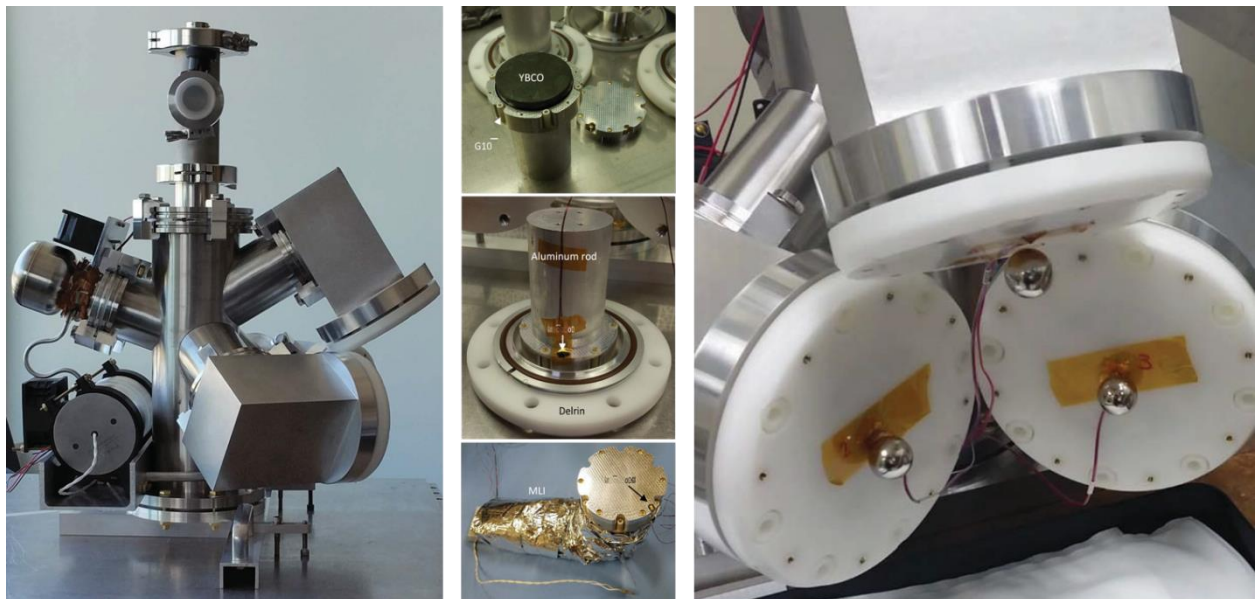
Figure 102: Images of the SROA assembly shown (left) assembled from the side, (center) in various stages of assembly, and (right) with levitating spherical magnets at the OSA equilibrium (these magnets are not the training magnets, which are bolted to the faces).
