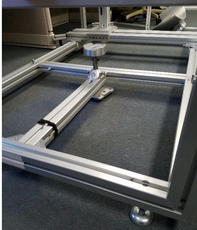
Figure 96: The base of the FA bolted together.
