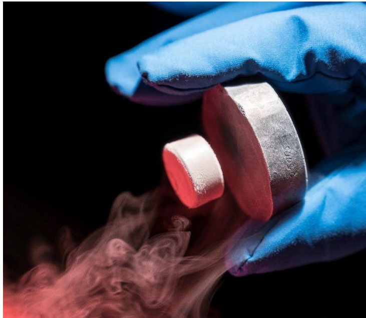
Figure 1: A Neodymium magnet (bottom) flux pinned to a YBCO superconductor disc (top). The YBCO was cooled below its critical temperature (~88K) in a bath of liquid nitrogen
