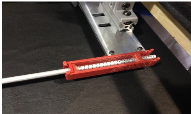
Figure 55: Spring boxes supply the force to impart an initial velocity on the air bearing
