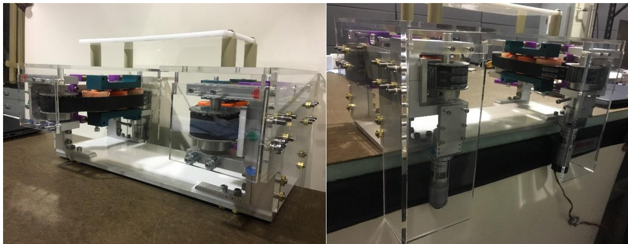
Figure 100: Initiator assembly launching mechanism, including safety covers and motors.
