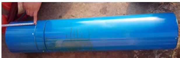
Fig. 11 High-frequency and low-amplitude axial impacting tool
