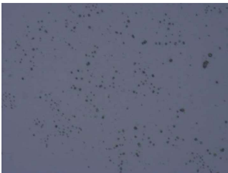
Figure [15]: Optical microscopy test showing the mid of our spin casting film. 20x zoom
